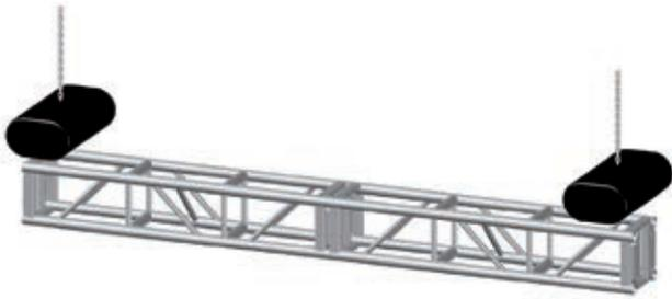
Figure 1: A span supported on each end—simple
