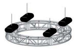
Figure 5: A circular indeterminate structure --not simple
